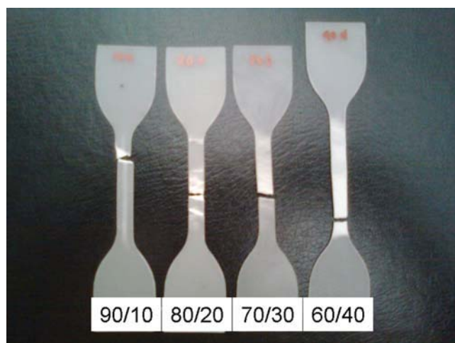
Figure 6 Visualization of break behavior of the tensile test specimens of PLA/impact modifier blends. [Color figure can be viewed in the online issue, which is available at wileyonlinelibrary.com .]
